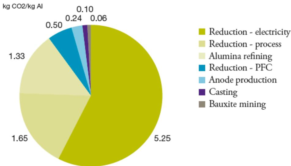
> Figure 9-2 Contributions to CO<sub>2</sub> emissions from the aluminium mine to ingot value chain
