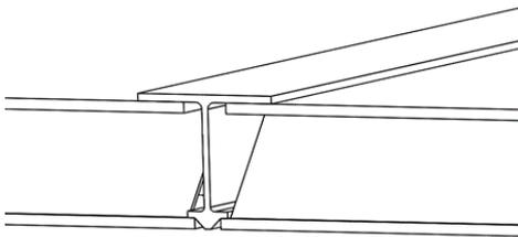
> *Figure 5-6 Weld support profile or transversal weld of side/bottom panels*
