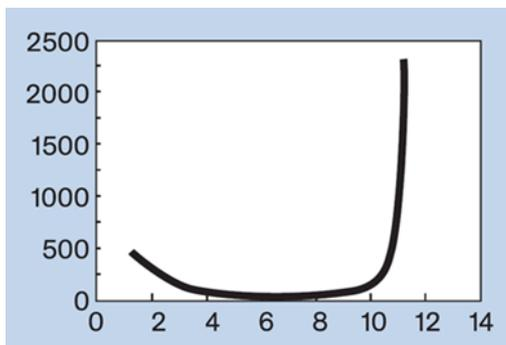
> Figure 3-17 Corrosion rate vs. pH
