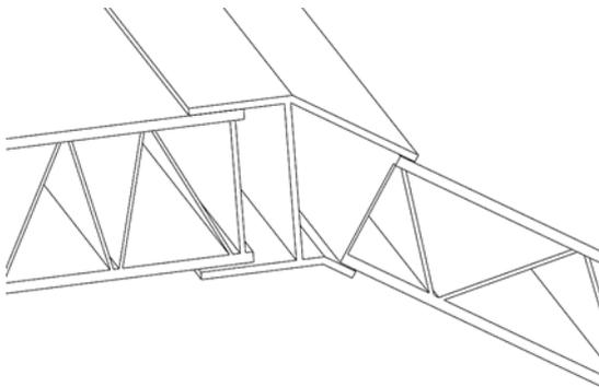
> *Figure 5-9 Joining lower side panel to bottom panel using joiner profile*
