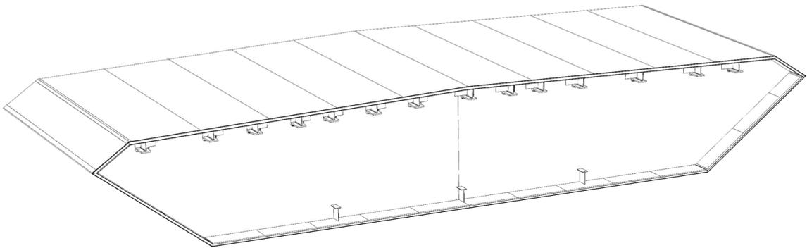
> *Figure 5-11 Main view of a girder section with bulkhead*
