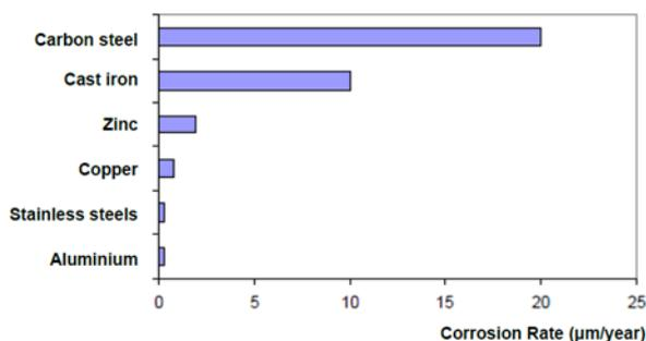
> Figure 3-18 Uniform corrosion in marine atmosphere
