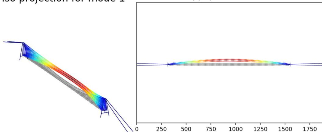
> Figure 6-5 The mode shape of the first eigenmode for the plate concept
