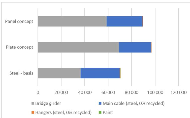
> Figure 9-6 CO<sub>2</sub> footprint based on Hydro European average material [ton CO<sub>2</sub>]
