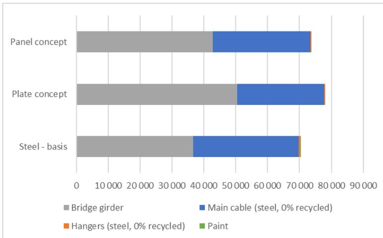
> Figure 9-5 CO<sub>2</sub> footprint based on Hydro 4.0 material [ton CO<sub>2</sub>]
