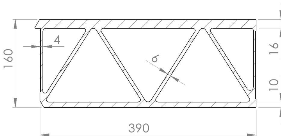
> Figure 5-21 Top deck panel toward joiner profile in bulkhead (right side)
