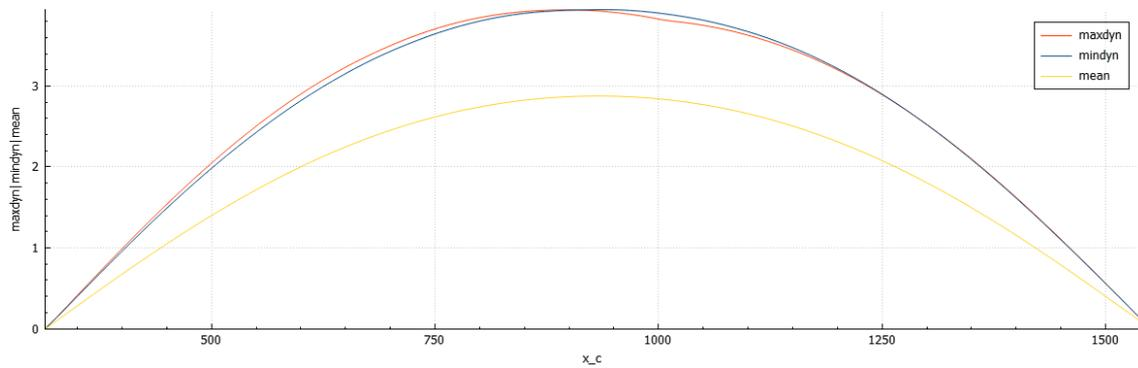
> Figure 6-4 Plate concept: Lateral displacement [m] of the bridge girder.
