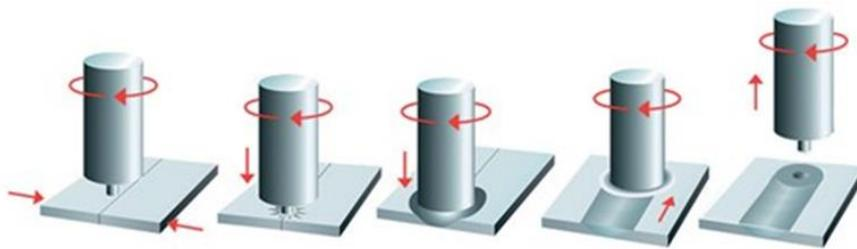
> Figure 3-12 Friction stir welding process (Hydro)
