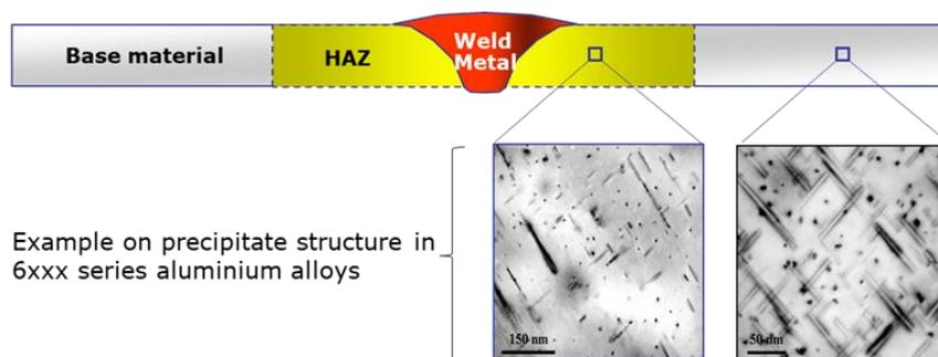
> Figure 3-10 Cross-section of welded joint
