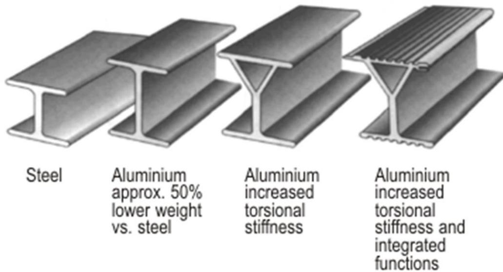
> Figure 3-16 Design of aluminium extrusion (AZOM)
