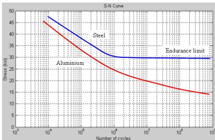
> Figure 3-15 Representative SN-curves for steel and aluminium
