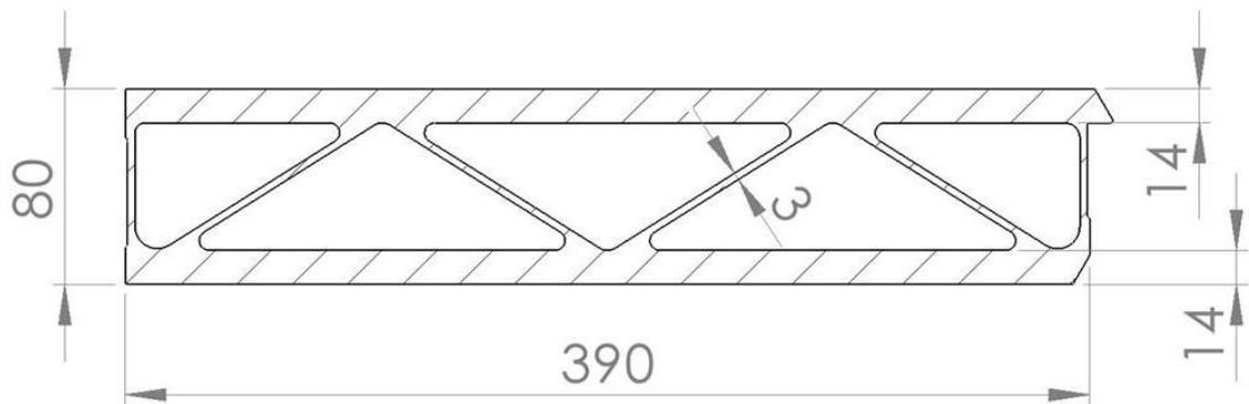
> Figure 5-23 Bottom and side deck panel towards joiner profile in bulkhead (right side)
