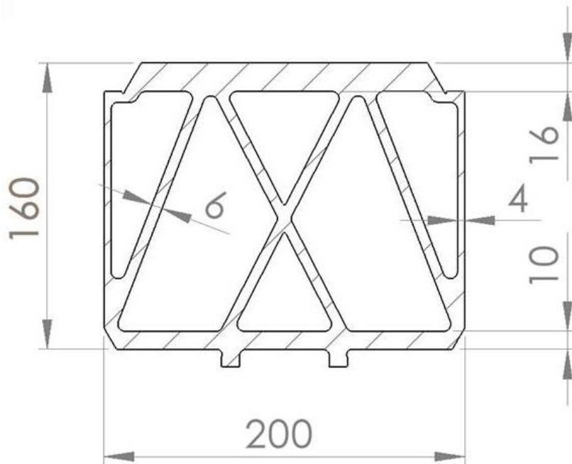
> Figure 5-24 Joiner profile between top deck and bulkhead, dimensions
