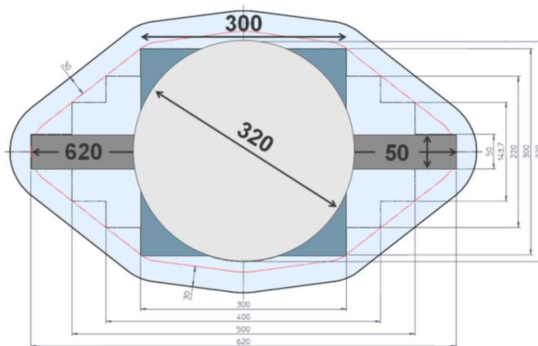
> Figure 3-9 Example of allowable profile dimensions at one extrusion plant (Hydro)
