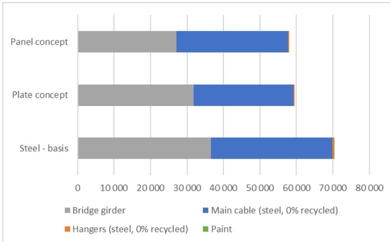
> Figure 9-4 CO<sub>2</sub> footprint based on Hydro 75R [ton CO<sub>2</sub>]
