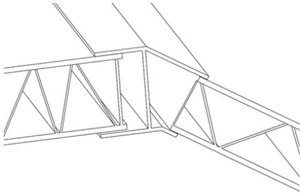
> *Figure 5-7 Joining deck panel to upper side panel using joiner profile*
