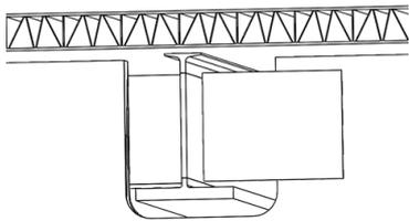
> *Figure 5-3 Shear plates to connect the I-beams to the bulkhead panels*
