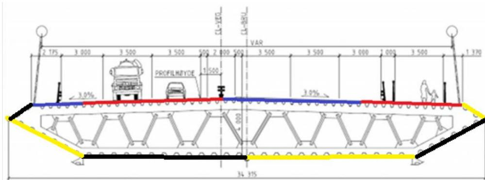
> Figure 5-28 Panel layout in the transverse bridge direction
