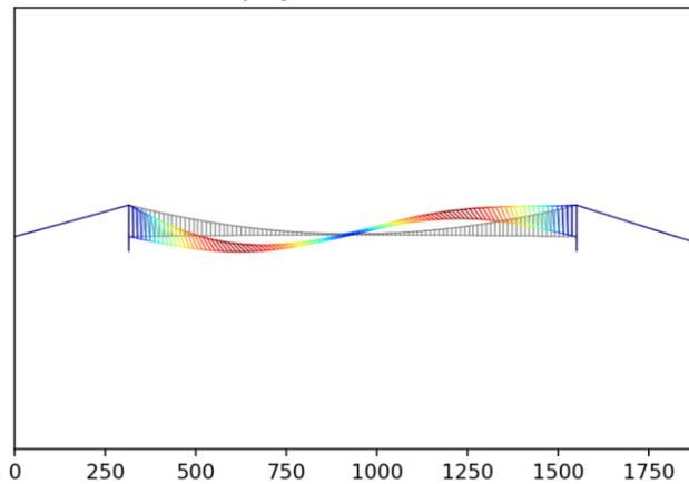
> *Figure 6-6 The mode shape of the second eigenmode for the plate concept*
